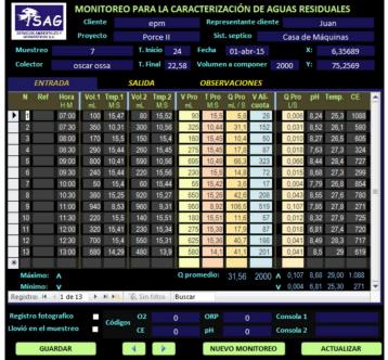
Platform on Tablet for characterization and monitoring of wastewater in the field; it allows automating the data processing and calculating the aliquot during composite sampling in real time.
